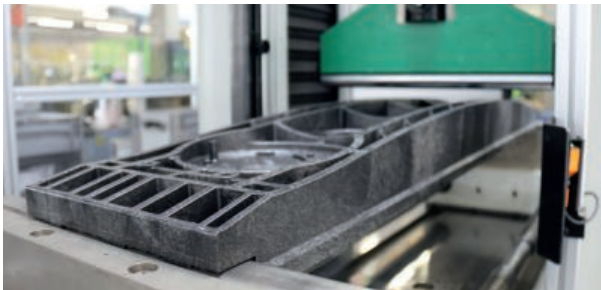
▲ 3-point static load hydraulic press at Langmatz in Oberau
