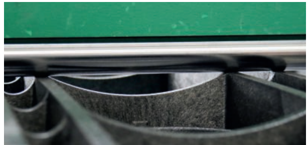
▲ Regular 3-point bending test every 2 hours
