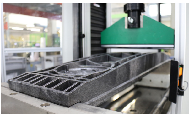
▲ 3-point static load hydraulic press at Langmatz in Oberau
