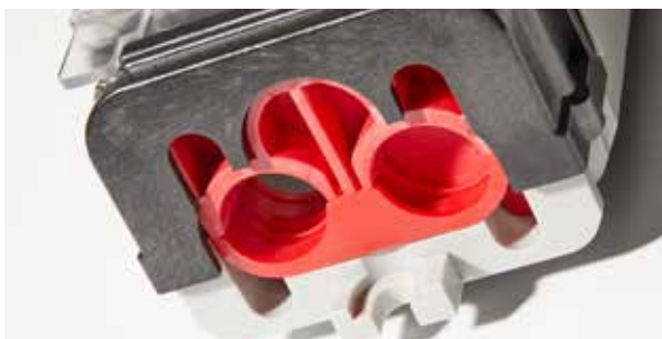
▲ Standard strain relief for 1 – 3 cables; cross-section from 7.5 – 19 mm
