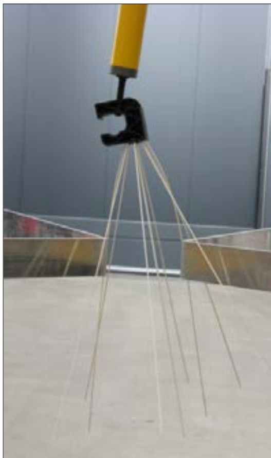
Electrical type approval test of an assembly rod for repelling tuft for a nominal voltage of up to 35 KV at Technical University in Dresden
